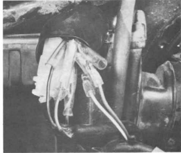
4.9a Disconnect the neutral switch and oil pressure switch leads
