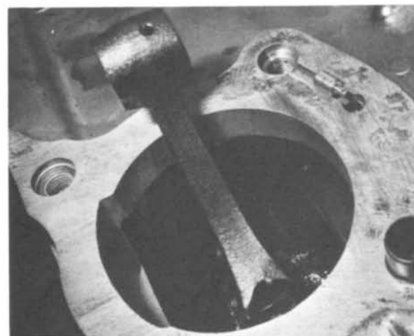
49.5 Insert the two locating dowels and position the two oil feed jets
