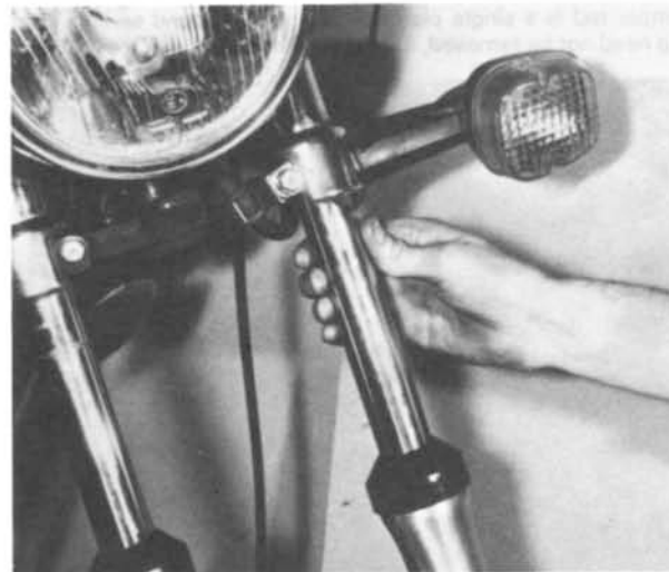
2.7c The fork legs can be withdrawn from the yokes
