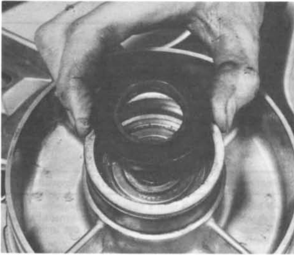
14.2d Do not omit to replace oil seal
