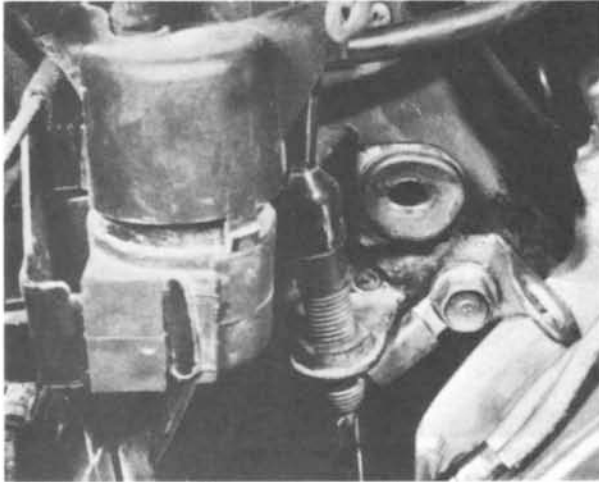
13.3b Adjustment of the stop lamp switch may be necessary
