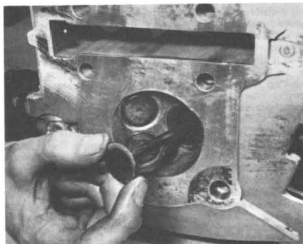
28.9b Lubricate the valve stem before insertion
