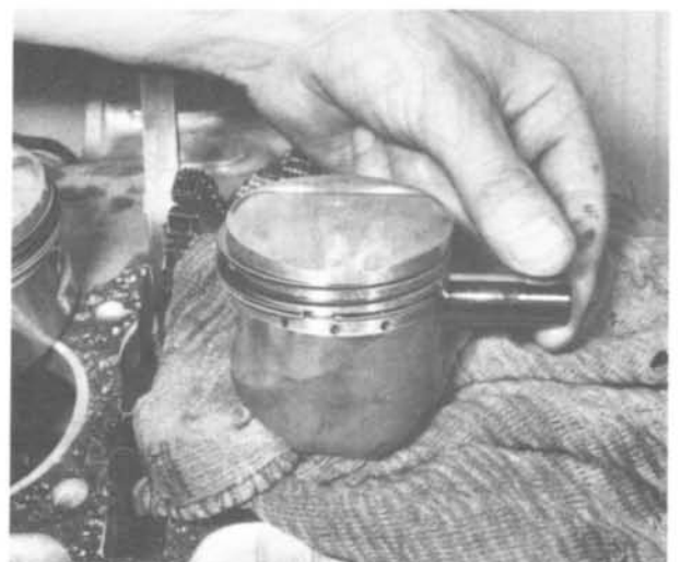
7.5b ... push out the gudgeon pin to free the piston
