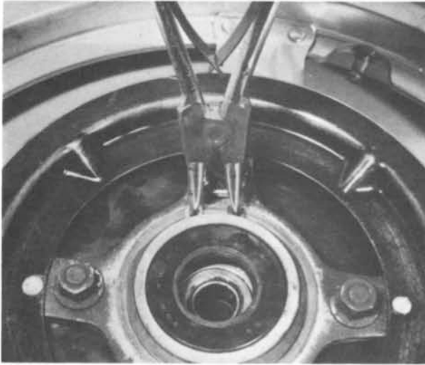
15.2b ... removal of the sprocket retaining circlip
