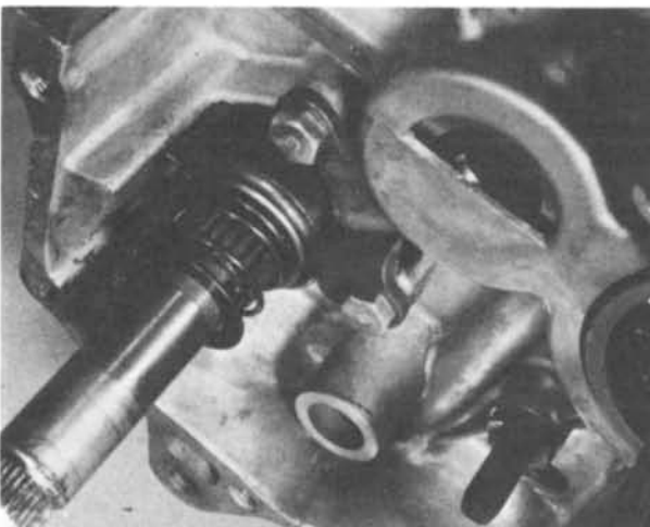
42.3a With kickstart pinion and shaft inserted ...
