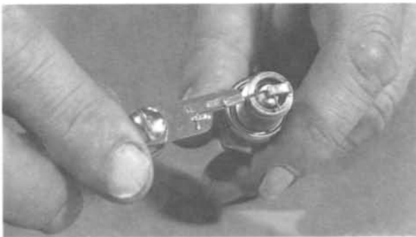
Spark plug maintenance: Checking plug gap with feeler gauges
