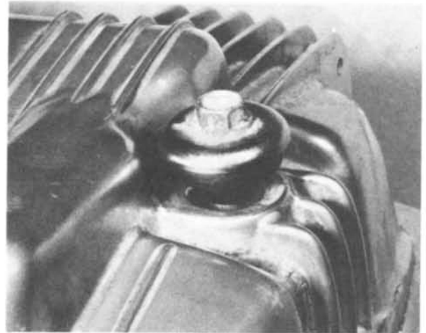
6.1 Loosen and remove the two head cover securing nuts
