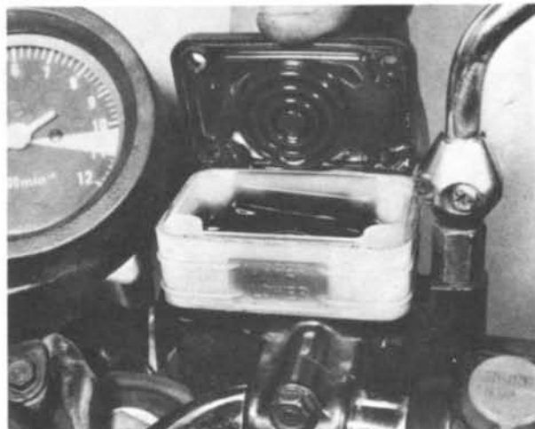
4.2 Brake fluid level should be between upper and lower marks
