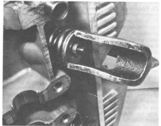
28.9d Compress springs to allow collet reinstatement
