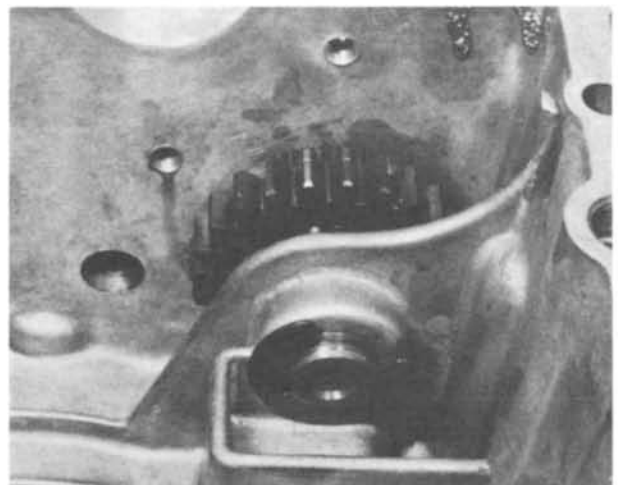
42.3b ... it is secured with the E-clip
