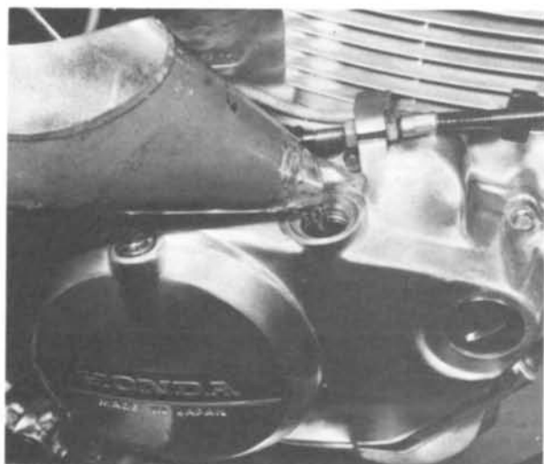
51.12 Refill the engine with the correct quantity of oil
