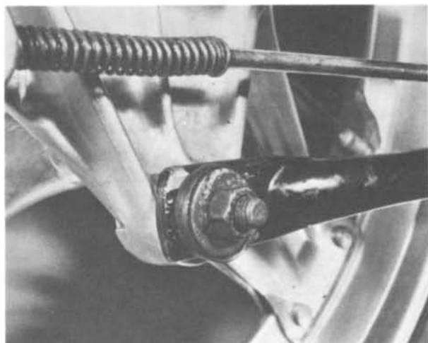
10.3 Detach the brake torque arm from the brake plate
