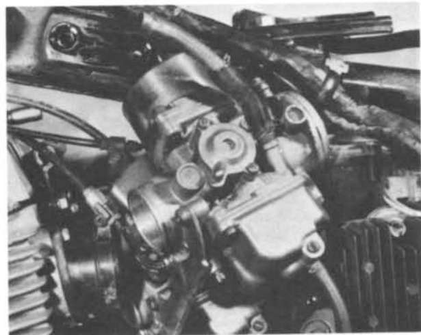
51.4b ... manoeuvre the carburettors into position
