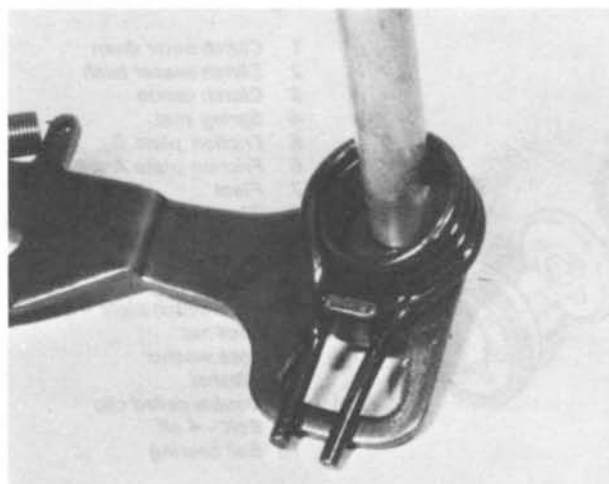
45.6a Fit centraliser spring only as shown
