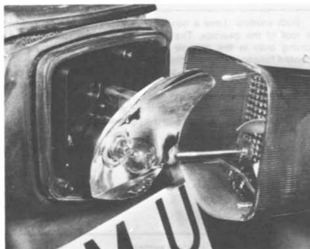
10.1 Stop/tail lamp lens is held by two screws as is ...
