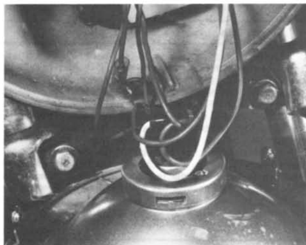
9.2a Headlamp bulb socket is a push fit
