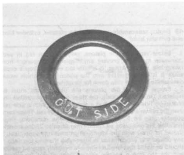
47.3b Note marks on centre nut washer; fit accordingly
