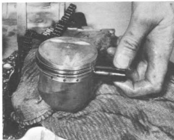
49.3a Lubricate small-end bearing before installing piston and gudgeon pin
