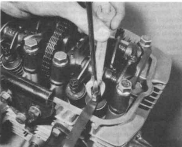
50.6 The feeler gauge should be a light sliding fit
