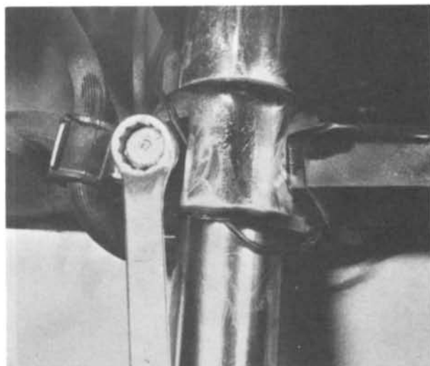
2.7b ... slacken the yoke pinch bolts
