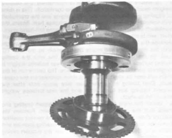
38.3b Rotate starter gear pinion in a clockwise direction to engage rollers
