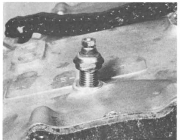
12.4 Unscrew and remove the neutral indicator switch
