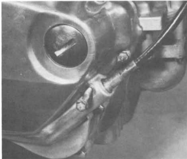
4.8c Tachometer cable is secured by a single bolt
