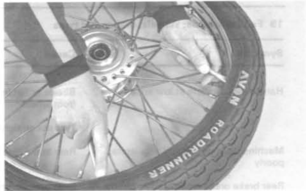
Use two levers to work bead over the edge of rim
