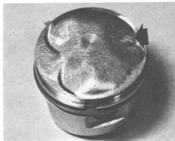
49.3b Fit piston with IN mark towards rear. EX mark (arrowed) forwards
