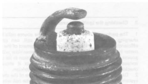
A blistered white insulator or melted electrode indicates over-advanced ignition timing or a malfunctioning cooling system. If correction does not prove effective, try a colder grade plug
