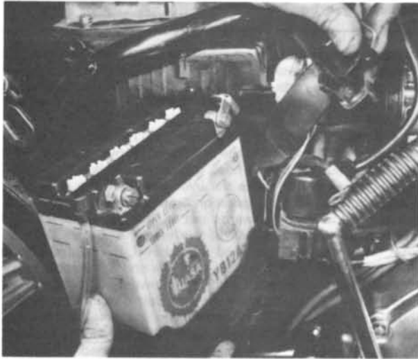
4.5 Detach securing strap and pull battery clear of carrier
