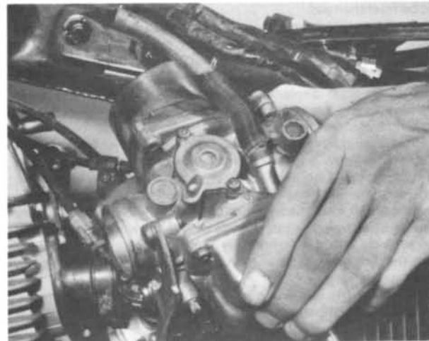
5.4a Carburettors can be removed as a unit and ...
