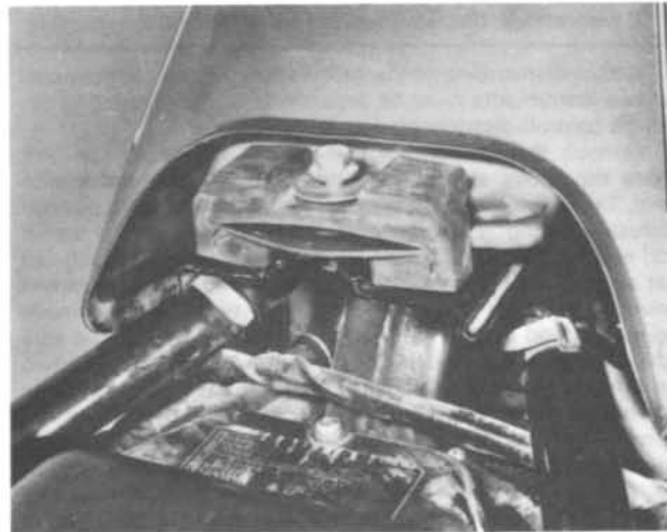
2.2 Single bolt retains fuel tank at rear
