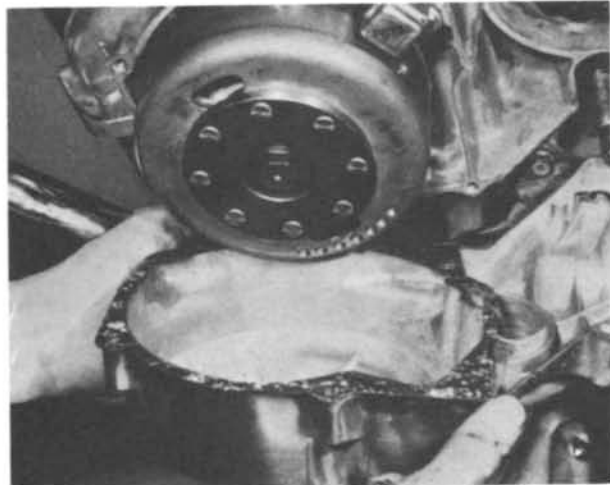
51.2 Refit the engine left-hand cover using a new gasket
